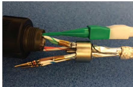
Figure 21: Inserting the wired contact in connector
