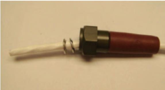
Figure 28: Sliding the backshell onto the cable
