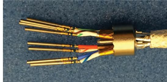
Figure 37: Inserting pairs through the metal follower
