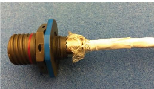
Figure 41: Returning the jacket to the connector
