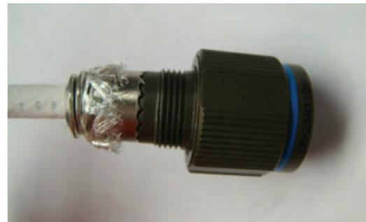
Figure 26: Placing the washers near the connector
