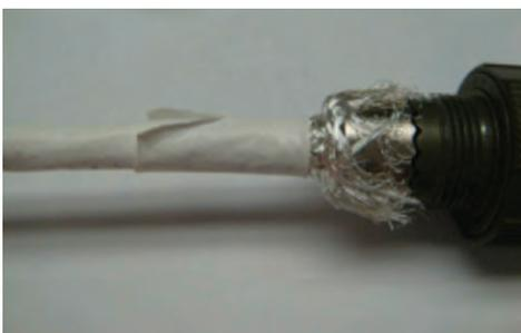
Figure 24: Returning the jacket to the connector
