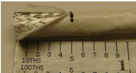
Figure 13: Slitting the cable jacket
