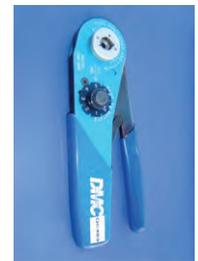
Figure 4: Crimpers (M22520/2-01 / AFM8)
