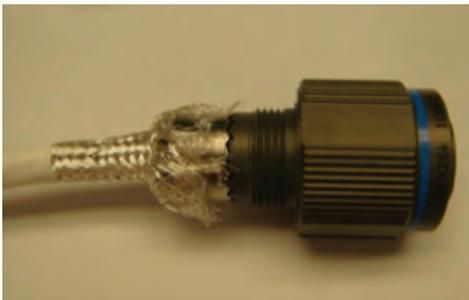
Figure 23: Folding the braid over the backshell
