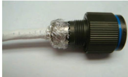
Figure 25: Trimming the excess braid material
