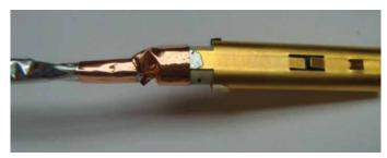
Figure 63: Taping the ears
