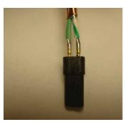
Figure 58: Soldering the twisted pair
