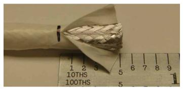
Figure 12: Slitting the cable jacket
