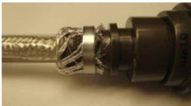
Figure 71: Attached Band-It® clamp
