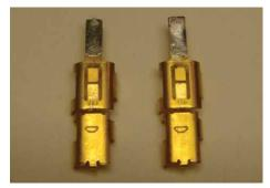
Figure 27: Tinning ears of outer body
