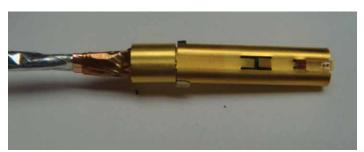
Figure 64: Positioning the ferrule
