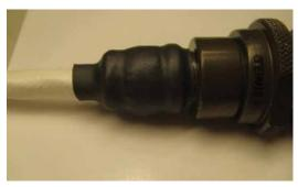
Figure 73: Shrinking tubing over backshell
