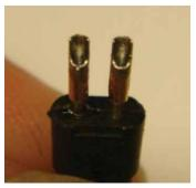
Figure 24: After degolding contacts
