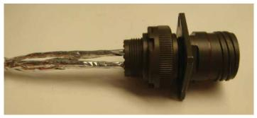
Figure 69: Connecting the grommet to the receptacle
