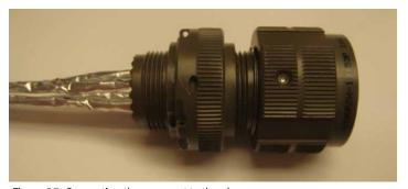
Figure 37: Connecting the grommet to the plug
