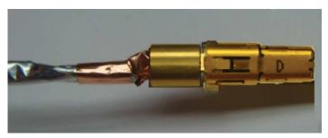
Figure 32: Positioning the ferrule
