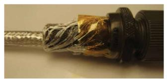
Figure 38: Returning braid to connector
