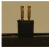
Figure 23: Before Degolding contacts
