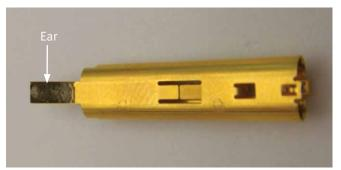
Figure 59: Tinning ears of outer body
