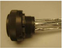
Figure 49: Pairs inserted in connector grommet
