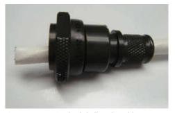
Figure 42: Inserting backshell on the cable
