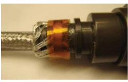
Figure 72: Wrapping Band-It® clamp
