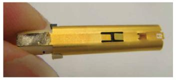
Figure 62: Locking outer body onto insulators
