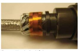
Figure 40: Wrapping Band-It® clamp
