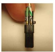
Figure 28: Attaching black rear insulator
