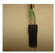
Figure 26: Soldering the twisted pair
