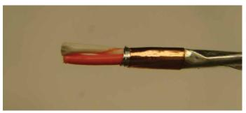
Figure 52: Removing polyimide tape and foil
