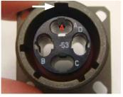
Figure 67: Front view with connector keyway
