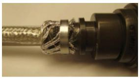
Figure 39: Attached Band-It® clamp
