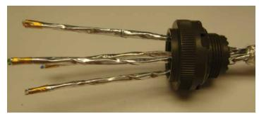
Figure 18: Positioning the grommet near the braid
