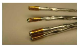
Figure 15: Taping each pair
