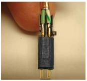
Figure 60: Attaching rear insulator
