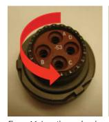
Figure 16: Inserting each pair into connector grommet
