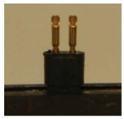
Figure 56: Before degolding contacts
