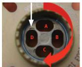
Figure 68: Rear view with insertion orientation
