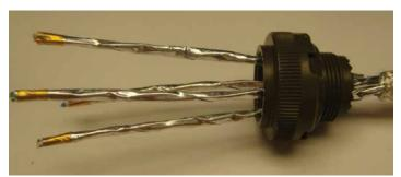
Figure 50: Positioning the grommet near the braid
