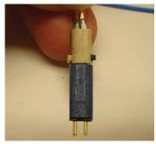
Figure 61: Attaching beige rear insulator
