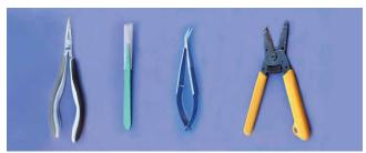
Figure 1: Needle nose pliers, scalpel, tweezer scissors, and hand strippers
