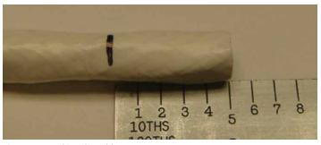
Figure 11: Marking the cable
