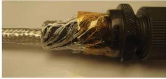
Figure 70: Returning braid to connector
