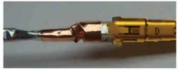
Figure 31: Taping the outer body ears
