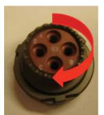
Figure 48: Inserting each pair into connector grommet
