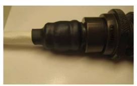
Figure 41: Shrinking tubing to backshell
