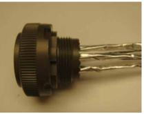
Figure 17: Pairs inserted in connector grommet
