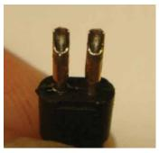
Figure 57: After degolding contacts
