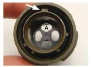
Figure 35: Front view with connector keyway
