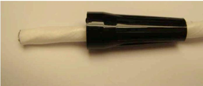
Figure 8: Attaching the connector cap
