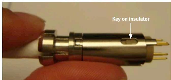
Figure 43: Insulator key for alignment
