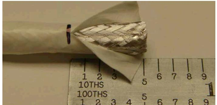
Figure 29: Slitting the cable jacket
