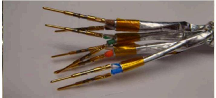
Figure 17: Stripping the pairs
