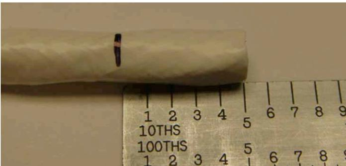
Figure 10: Marking the cable
