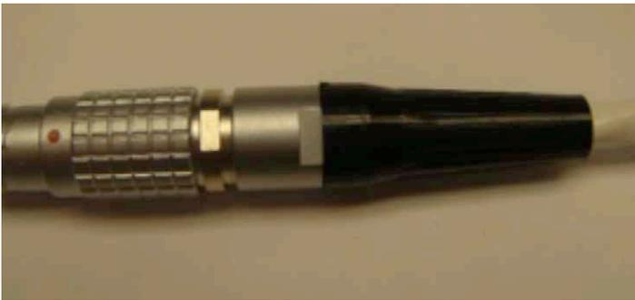
Figure 44: Installing the connector cap on plug end
