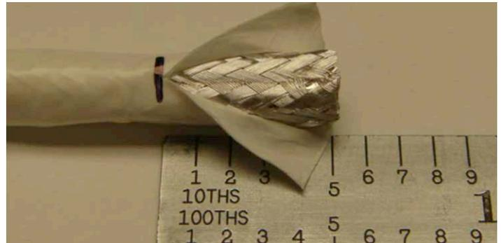
Figure 11: Slitting the cable jacket
