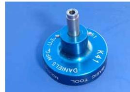
Figure 4: Socket positioner (K41)
