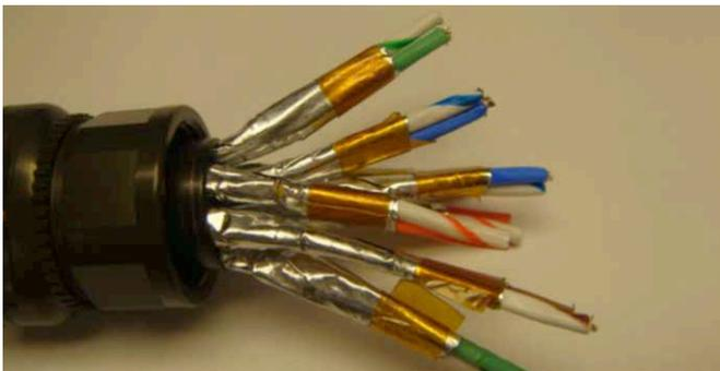
Figure 22: Removing the foil
