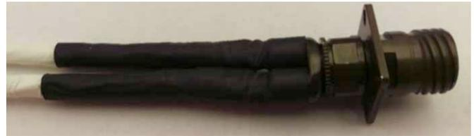
Figure 50: Covering the receptacle with TAT material
