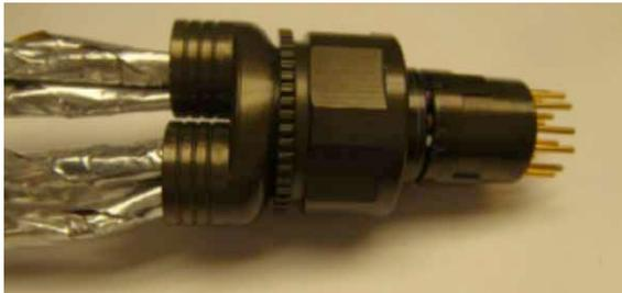
Figure 28: Top and bottom inserts together
