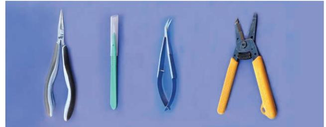
Figure 1: Needle nose pliers, scalpel, tweezer scissors, and hand strippers
