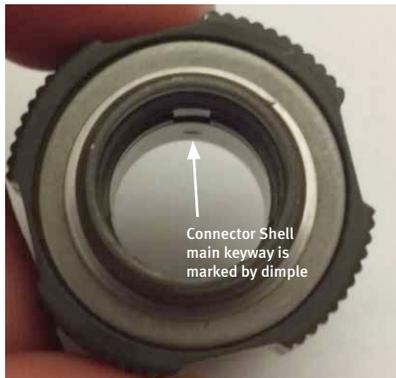
Figure 29: Inserting connector shell on cable
