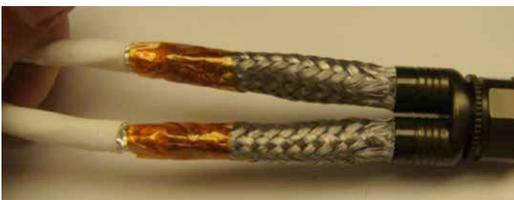
Figure 47: Taping the braid
