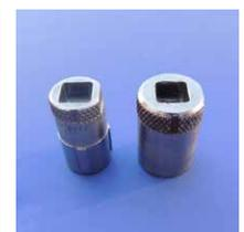
Figure 11: Torque adapters
