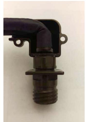
Figure 52: Attaching right-angle backshell
