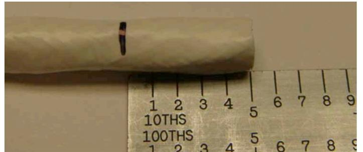
Figure 31: Marking the cable
