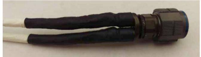
Figure 49: Covering the plug with TAT material
