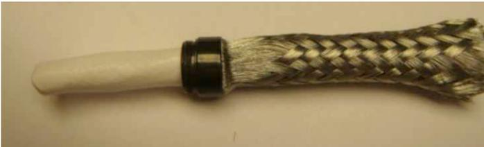
Figure 14: Inserting cable into braided shield
