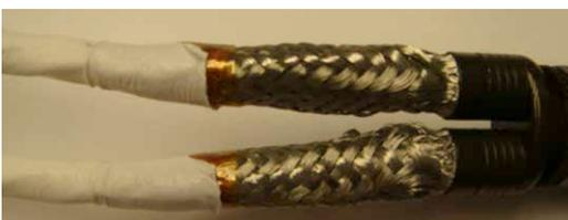
Figure 48: Repositioning the outer jacket
