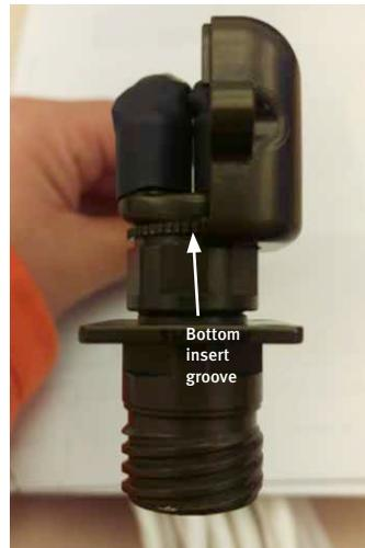
Figure 51: Attaching backshell
