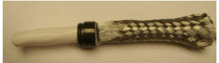
Figure 30: Inserting cable into braided shield
