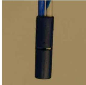
Figure 41: Inserting pair into insulator
