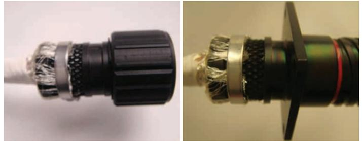
Figure 45: Trimming excess braid on plug
