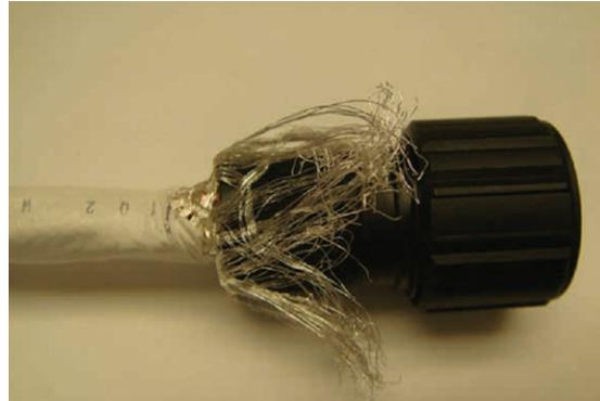
Figure 26: Returning the outer jacket
