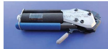
Figure 5: Clamp tool (Tie-Dex® II)
