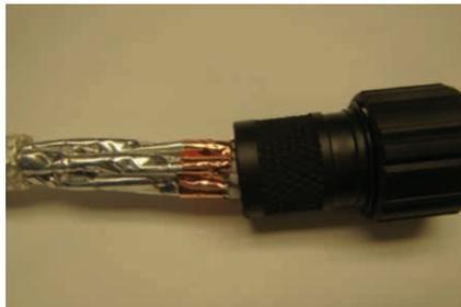
Figure 24: Inserting primaries into the connector
