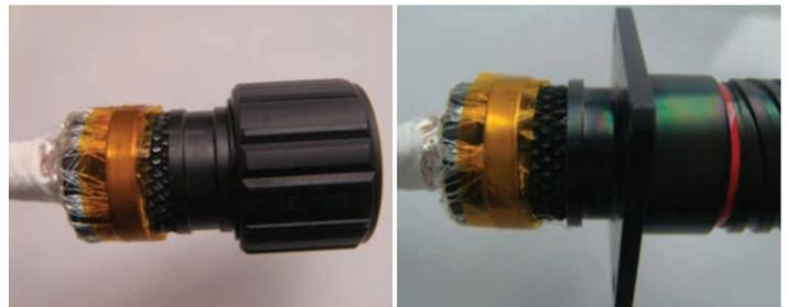
Figure 47: Taping the plug
