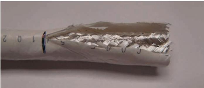
Figure 12: Slitting the cable jacket
