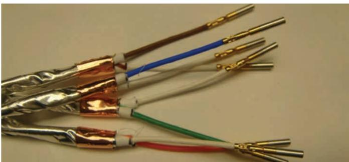
Figure 38: Stripping and crimping primaries
