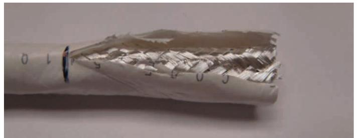
Figure 28: Slitting the cable jacket
