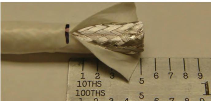
Figure 10: Slitting the cable jacket
