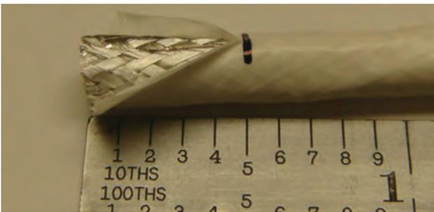
Figure 27: Slitting the cable jacket
