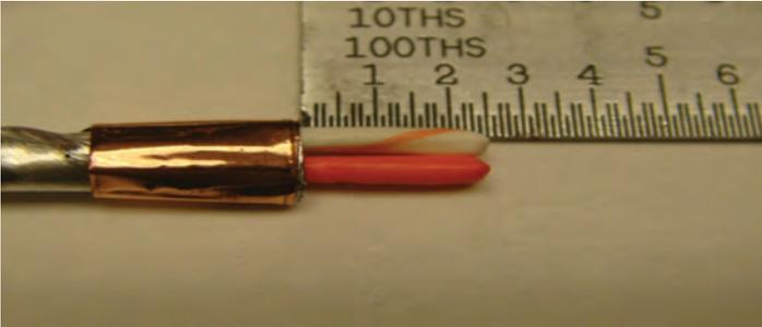
Figure 14: Removing the foil edge
