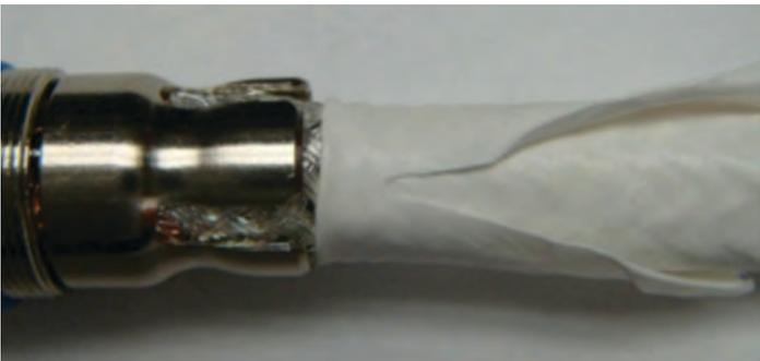
Figure 39: Returning the outer jacket
