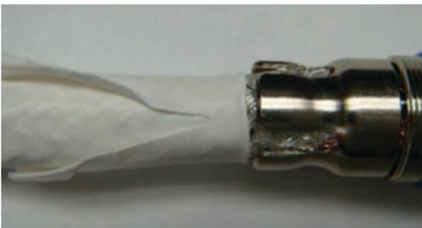
Figure 22: Returning the outer jacket
