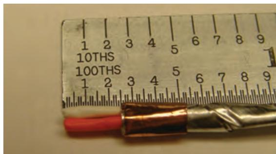
Figure 31: Removing the foil edge
